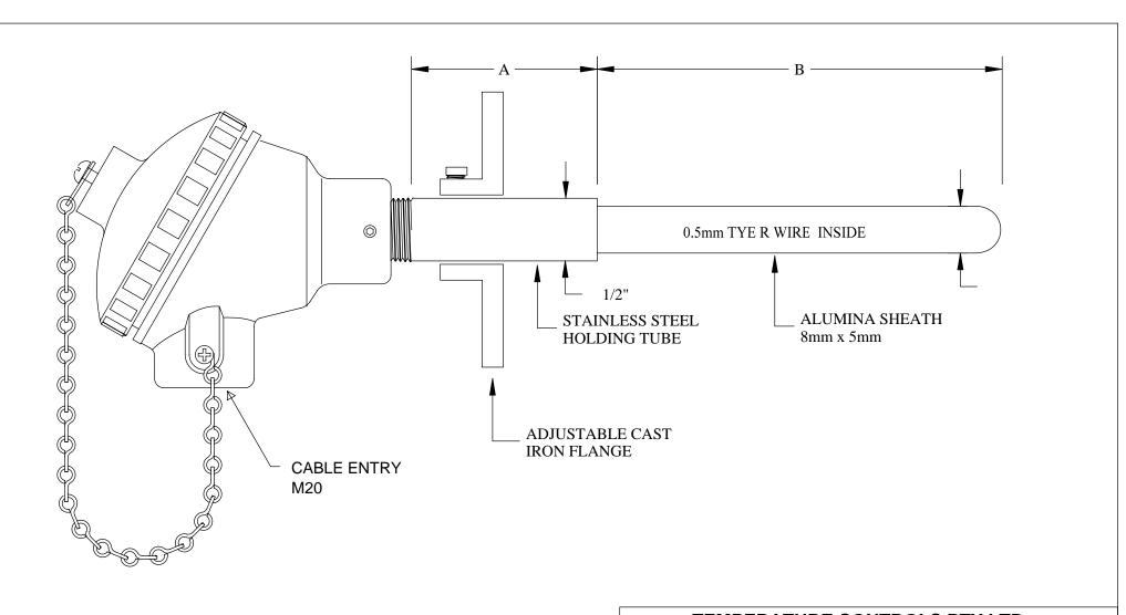
TYPE R THERMOCOUPLE LARGE TERMINAL HEAD IP65 STAINLESS STEEL SUPPORT TUBE ALUMINA SHEATH
